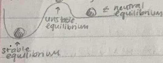
In the absence of friction, a small displacement of a system from a position of stable equilibrium causes the system to oscillate.
