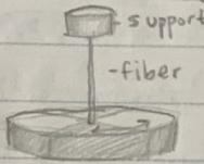
A torsional oscillator is an example of rotational rather than translational displacement. If the disk is twisted, elastic potential energy is stored in the fiber. When the disk is released it oscillates its energy back & forth between elastic PE & rotational KE.
