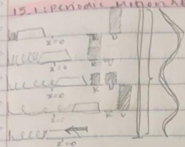
The cart does not stop at  $x=0$  because its potential energy is 0 but its kinetic energy is not 0. When  $KE = 0$ , direction reverses. This will happen indefinitely unless energy is dissipated. Dying out of periodic motion due to dissipation of energy = damping.
